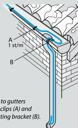
Fitted to gutters using clips (A) and mounting bracket (B).
